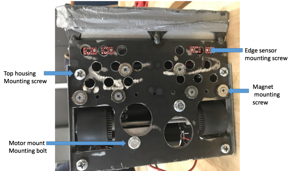
Figure 7.8: Base fastener location reference
