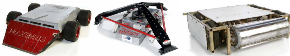
Figure 4.1: (Left to right) – Wedge, horizontal spinner, and drum robot designs [7].
