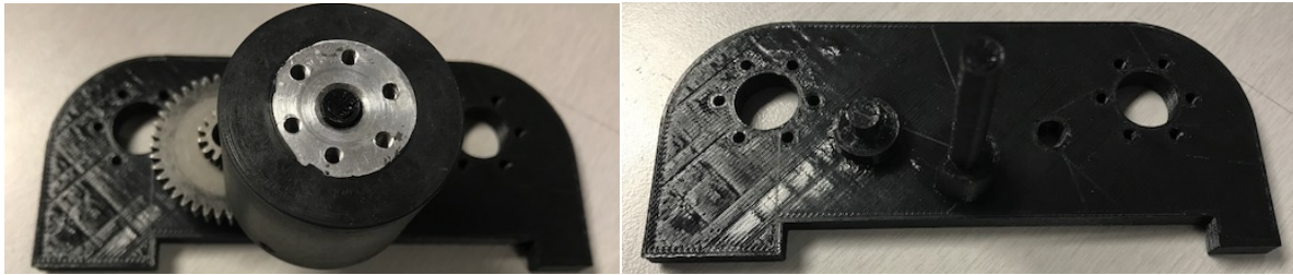
Figure 7.16: Gear and wheel mounting components
